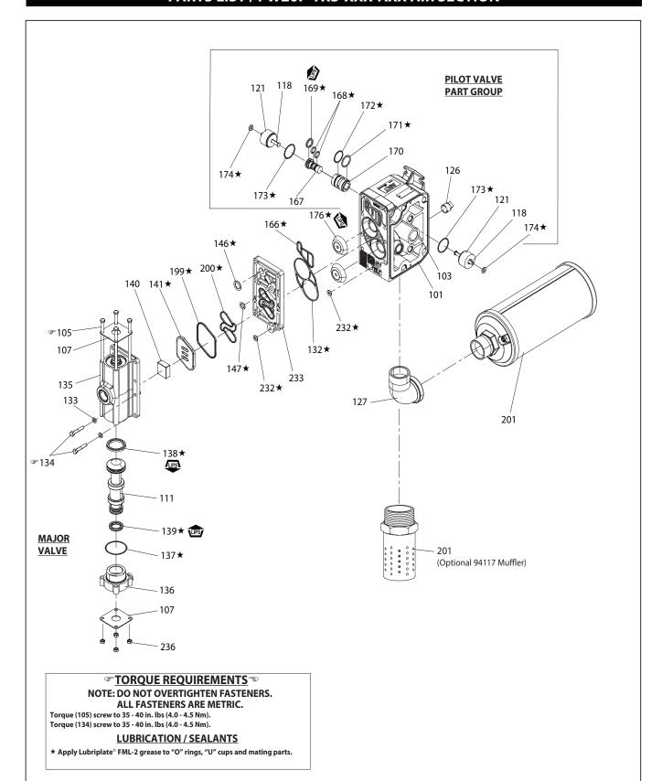
A replacement Major Valve Service Assembly is available separately, which includes the following: For Standard Pump Modles:
