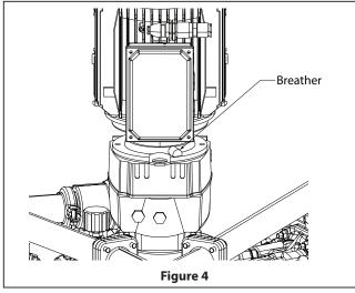
The hazardous motor gearbox will require the installation of an oil expansion tank.
