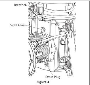
The ordinary motor gearbox will also need to have a breather installed after installation to the pump.
