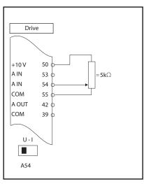
**NOTE**: Once parameter 420 is set to "[6] Analog in 54", this will be the source of the torque limit setting whether the VFD is in "Hand On" or "Auto On" mode. The pump will not operate if there is no signal on A54 or if the signal is too low.
