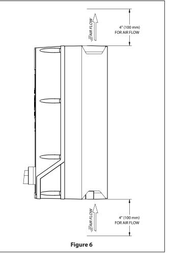
Accessory Option: Stainless Steel Backplate for use when the VFD cannot be mounted directly to a flat surface for proper cooling. See section 1.2 to confirm VFD frame size.
