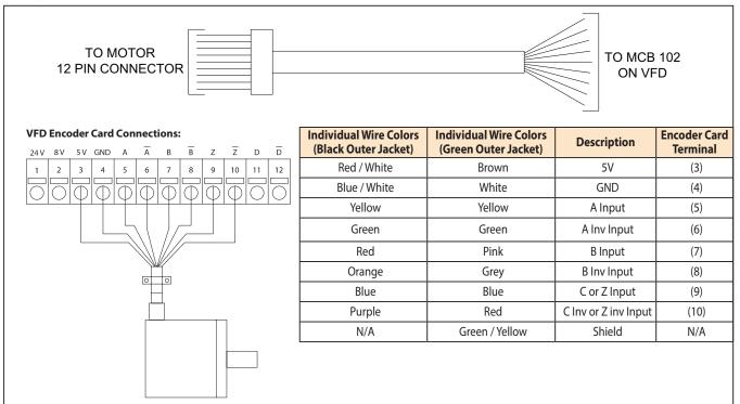
NOTE: Ensure the cable shielding is grounded to the VFD frame.
