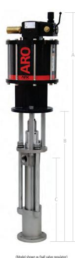
Materials: Caulking, Inks. Mastics, Heavy Lubricants, Sealants **Pump Specifications** Ratio 20:1 Stroke (double acting) 6" (15.24 cm) Material Inlet Flange Mount
