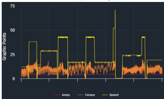
Runtime and Pump Speed Monitoring Graphic
