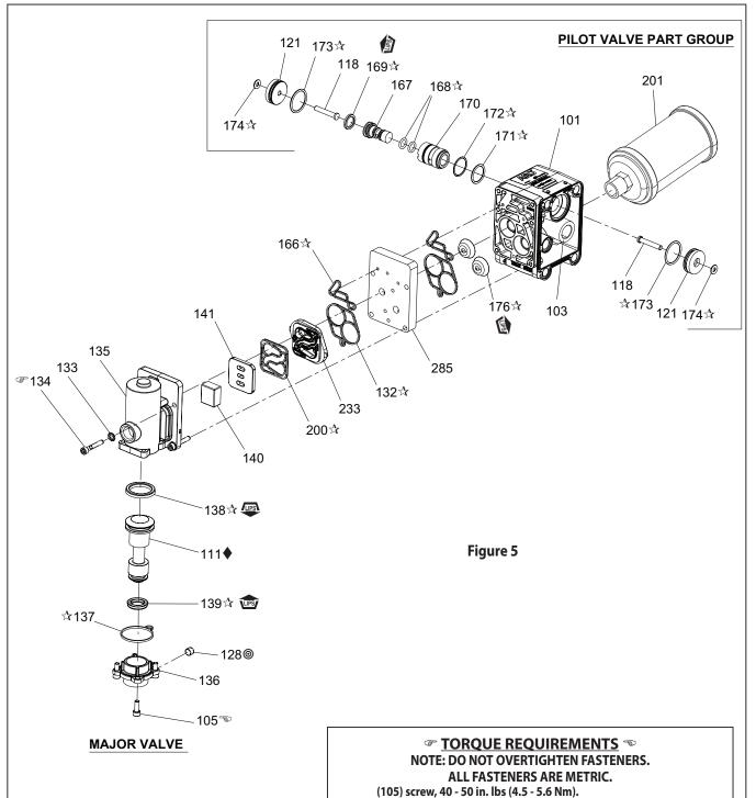
(105) screw, 40 - 50 in. lbs (4.5 - 5.6 Nm). (134) screw, 40 - 50 in. lbs (4.5 - 5.6 Nm).
